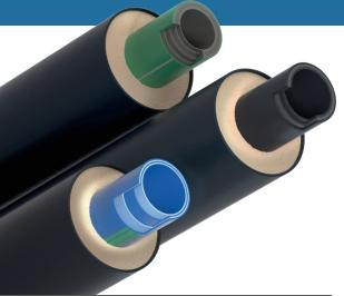
The POLYMELT pre-insulated piping systems are insulated with PUR rigid foam and enclosed with a PE jacket pipe. All medium pipes can be made of POLYMELT fiber pipes from the Ecosan and Mechanical product lines.
