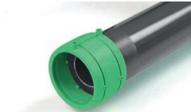
Do not touch peeled pipe ends again and protect them from new contamination – e.g. put a clean plastic bag over them. Weld within 30 minutes after the peeling process.
